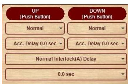
**Normal:** The relative relay is "ON" when the pushbutton is pressed and held, and relay is "OFF" when the pushbutton is pressed.
